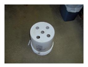
Then you drill out 4 evenly spaced 3/8" holes on the top edge of the bucket and run 2 pieces of rope through the holes, each rope about 6'. Run the rope through a D ring swivel (costs about \$3 at the local hardware store). Tie the ropes so that the knots are on the outside of the bucket.
