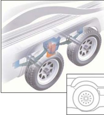
The MOR/ryde RE system works with the existing leaf springs and axles, but replaces the steel leaf spring equalizer. It isolates and absorbs road shock and increases the dynamic travel of the leaf spring suspension.
